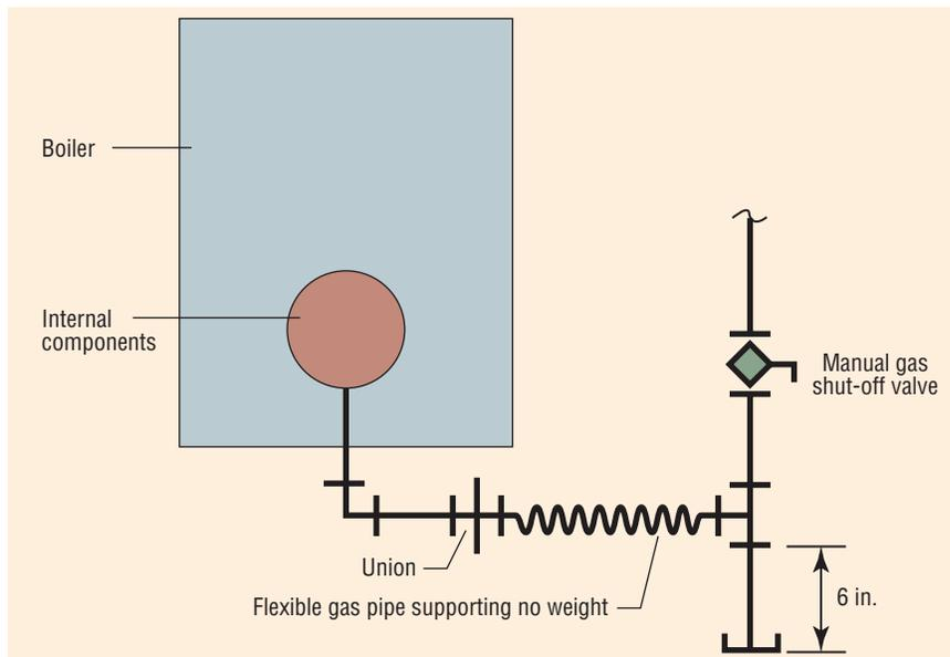
FIGURE 1. Boiler gas piping.
